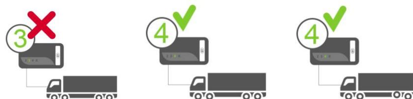
To change the number of axles, press the push-button longer than 2 seconds until the correct number of axles is indicated. To check the OBU status including the current number of axles, press the push-button once for less than 2 seconds. The light indicator should flash green.
